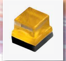
Cree X-lamp XQ-B / XQ-D Seramik tabanlı en küçük Power LED 1.6 x 1.6 mm XQ-D, min. 130lm @ 350mA, Maks. 700mA XQ-B, min. 52.5lm @ 150mA, Maks. 300mA
